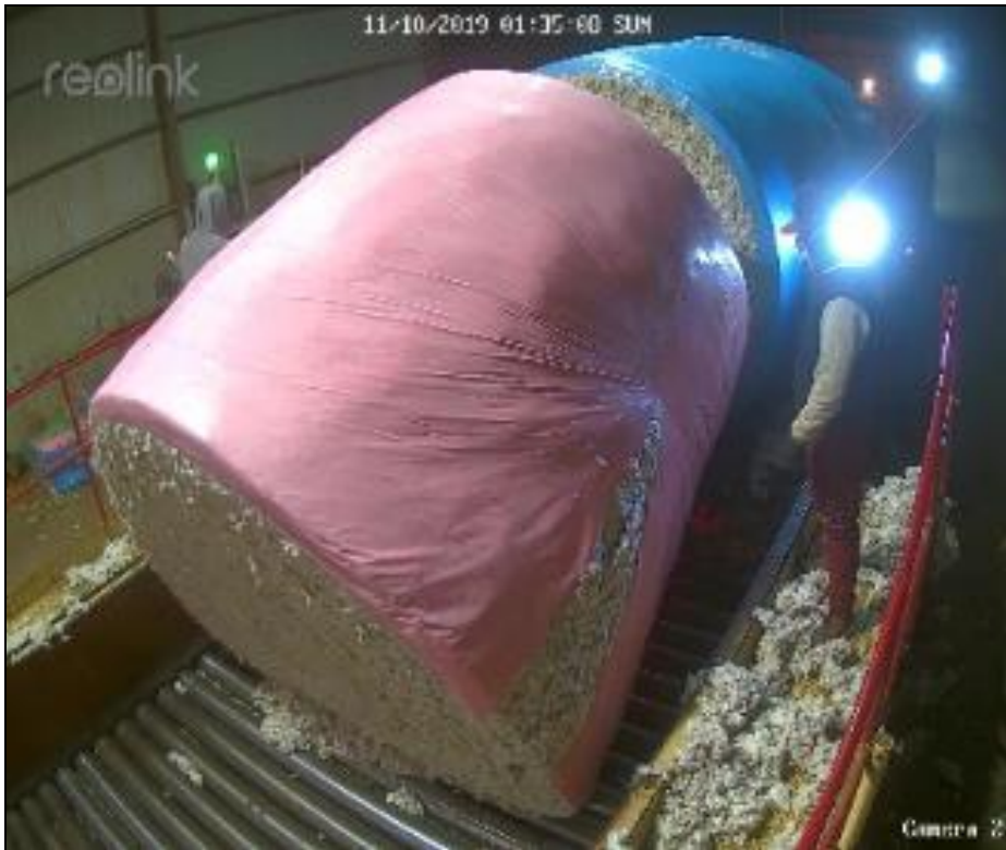
Figure 9. Image taken from the unloading video captured for the pink module in view (camera 2). The video showed that the module fell backward onto the truck and module feeder bed trapping a portion of the wrap material underneath the cotton.
