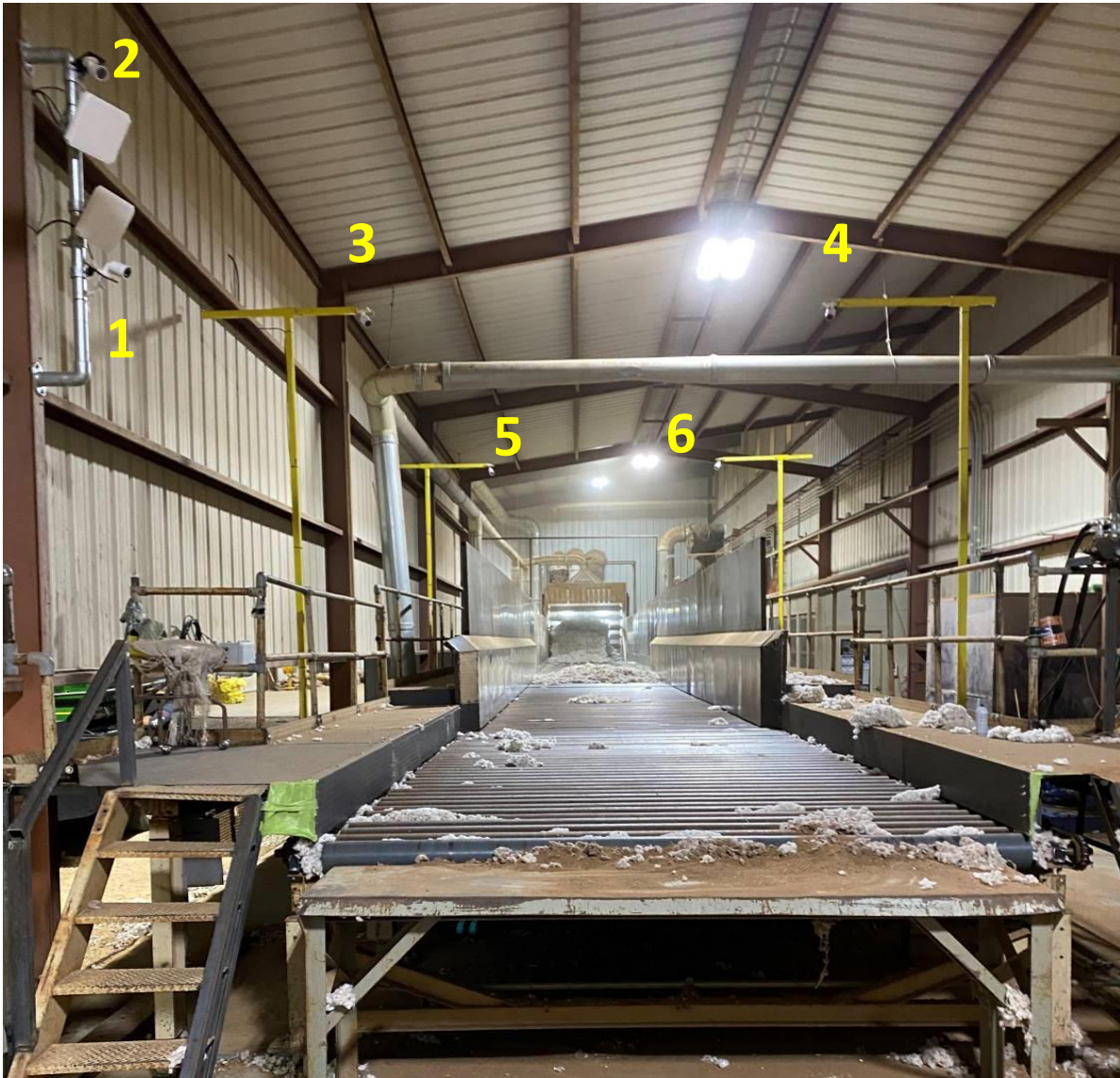
Figure 6. Photo showing numbered camera positions used on the module feeder at Gin B in 2020. RFID antennae are located between camera positions 1 and 2.
