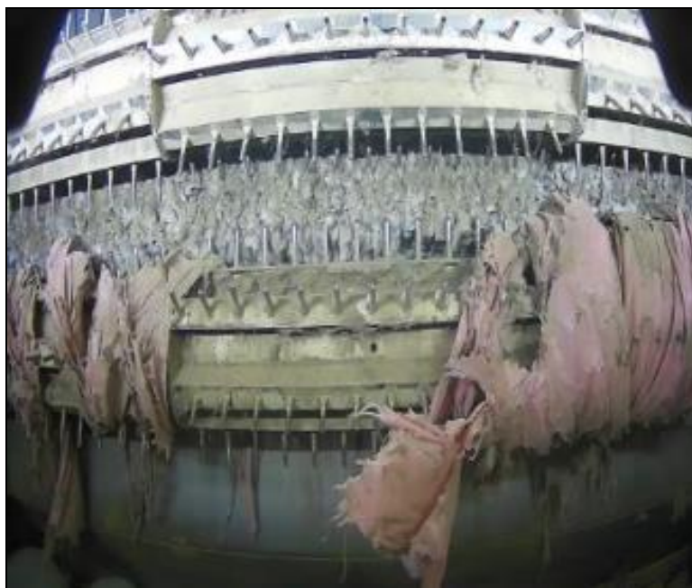
Figure 7. Lower dispersing cabinet camera still image of pink plastic caught on bottom dispersing cylinder.
