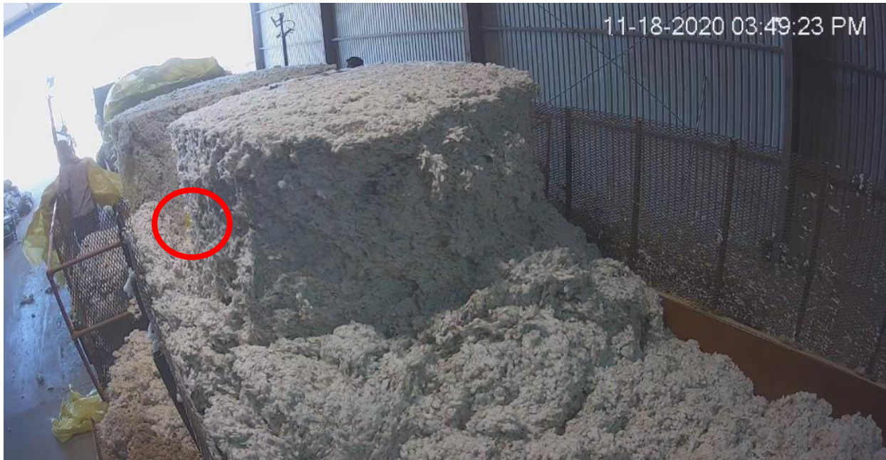
Figure 13. Still image from the unloading video captured for module SN 19410229688 showing piece of yellow plastic remaining in cotton between modules after wrap was removed from the top of the module.
