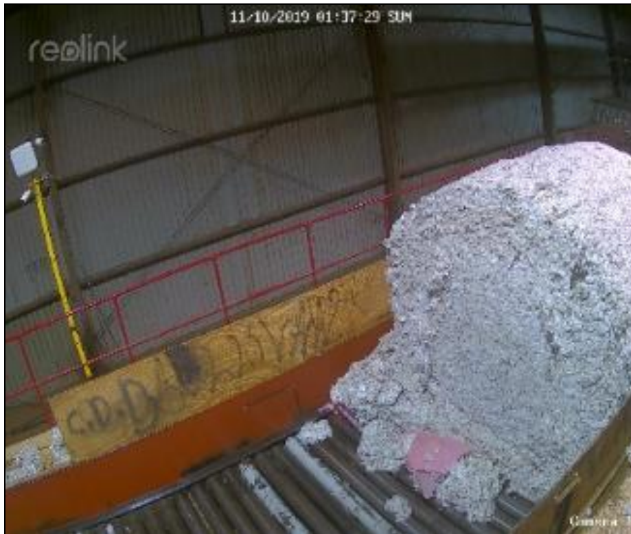
Figure 10. Image taken from the module unloading video (camera 4) showing plastic remaining under the cotton after attempts to remove the trapped material.
