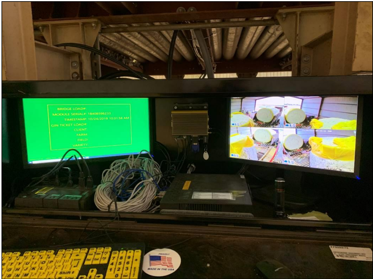
Figure 4. Photo of the enclosure box mounted below the module feeder bed at Gin A that housed the electronics and displays for the RFID Feeder Bridge (left display) and NVR (right display) systems.
