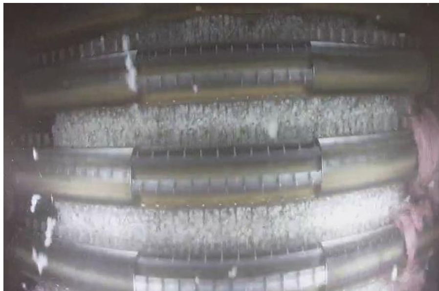
Figure 1: Module feeder image capture by inspection system with pink plastic on dispersing cylinders.
