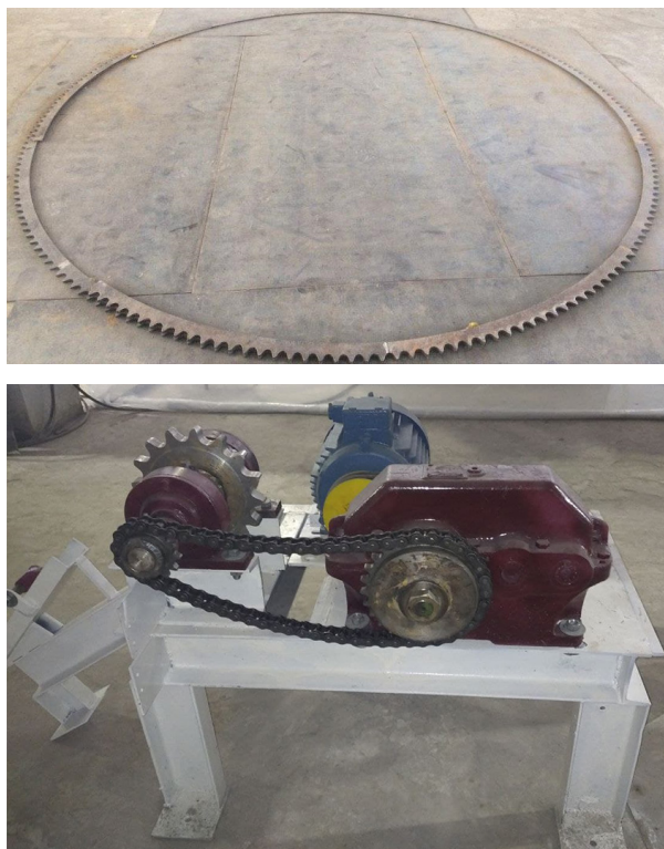
Figure 5. Fragment of the manufacturing process of the ring gear and drive chain drive.
